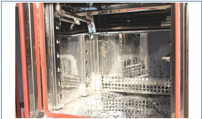
Water Spray System
